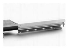
15.3 Attach the slack tray with the nuts and bolts. Tighten the nuts. Re-install the bottom tray by aligning the tray pins with the bottom holes of the bracket. Squeeze tray pins and slip tray into the bracket.
