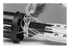
16.5 Carefully bend the intertray jumper tube to the appropriate tray and secure to the splice tray with two tie-wraps.
