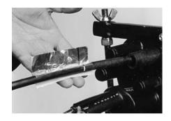
11.10 Slide the cable seal over the port. Shrink the cable sleeve on the base side with the recommended hot air gun device. Use the reflector to ensure heat distribution around the outlet. Shrink sleeve until the green thermo-indicating paint is converted to black.
