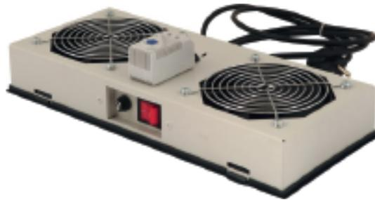
Fan Modules for wall Mounting, Ready pre-installed, plug-in and run style , with on/off switches or with analog thermostat and plugs. Each Fan has an air flow capacity of 2,3-3 cbm/min. Fan Technical data : 18/17 W, 220/240 VAC, 50/60 Hz, 013/0,11 A,2300/3000 rpm 42 dB noise level, Fan life: 10.000 hours
