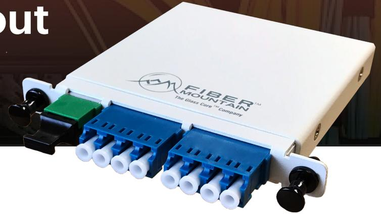
Fiber Mountain J-Series breakout panels provide all front-facing connectivity. The panel is modular with room for 8 MPO-to-LC cassettes in a 1 RU frame. Cassettes include Type A and Type B mapped QSFP breakout for 40G, 100G and 400G applications, and are available with Single Mode and Multimode fiber.
