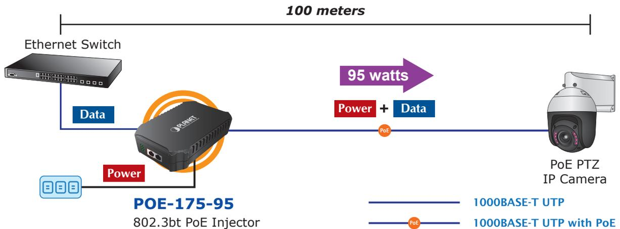
*Installation of 802.3bt PoE Injector and Splitter*
