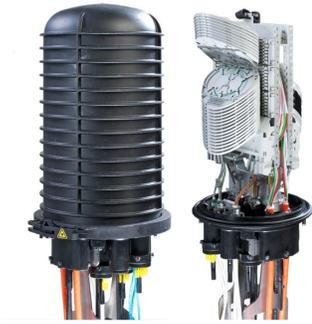
FIST™ GC02 Fiber Optic Splice Closure, Heat Shrink Cable sealing, size BC, no pre-installed fiber trays, 16 ports without grounding,
